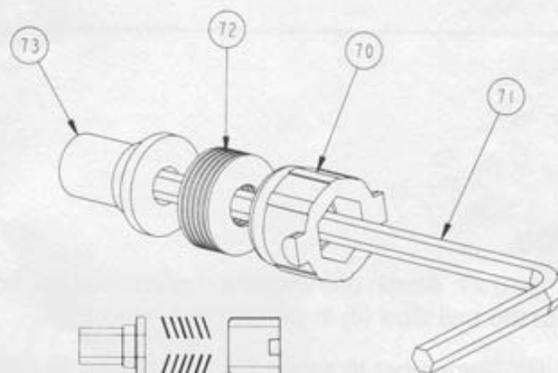
Bevelled washers should face this direction
